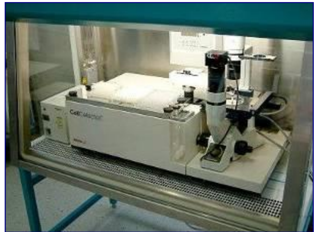
Fig.14 The CellCelector can be placed in a flow box for increased safety of cell cultures
