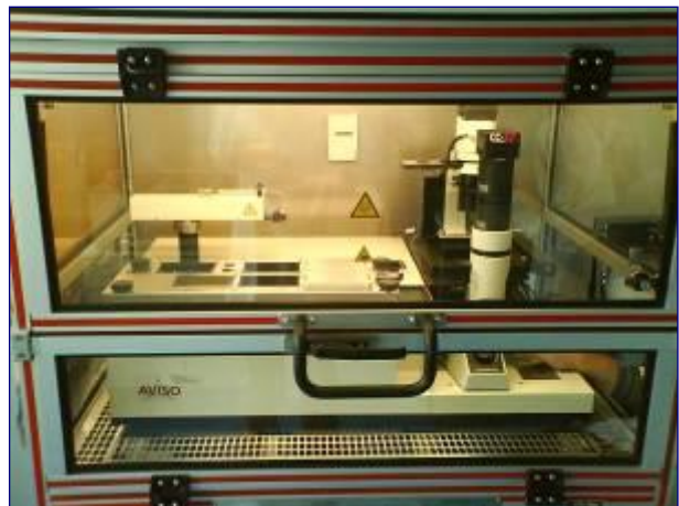
Fig. 15 The CellCelector is placed in the ALS Incubator FlowBox with high CO 2 -atmosphere and heated environment (37°C), especially useful for long-term experiments and primary cell cultures.
