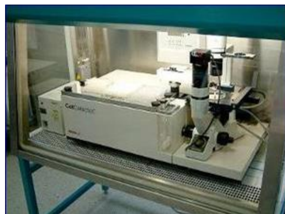
Fig.21 The CellCelector can be placed in a flow box for increased safety of cell cultures
