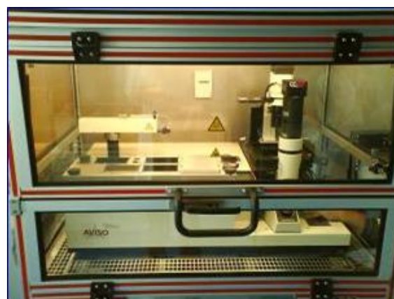
Fig. 22 The CellCelector is placed in the ALS Incubator FlowBox with high CO 2 -atmosphere and heated environment (37°C), especially useful for long-term experiments and primary cell cultures.
