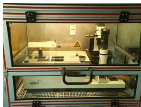
Fig. 24 The CellCelector is placed in the ALS Incubator-FlowBox with high CO 2 -atmosphere and heated environment (37°C), especially useful for long-term experiments and primary cell cultures.
