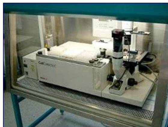
Fig. 23 The CellCelector can be placed in a flow box for increased safety of cell cultures
