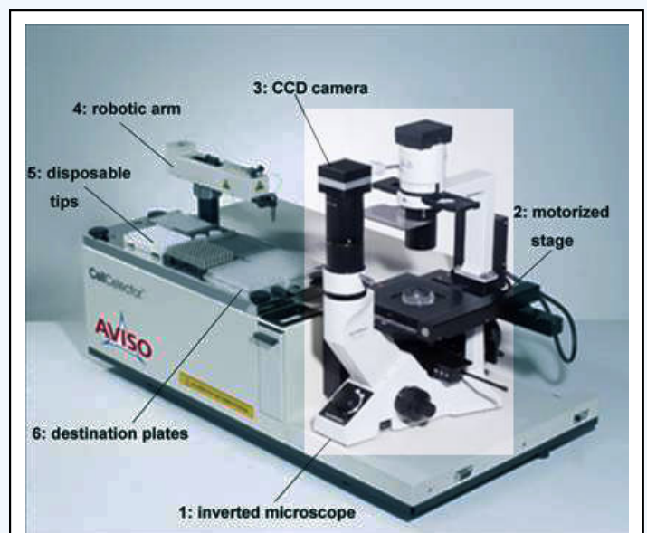
Figure 1: Assembly of AVISO's CellCelector™, robot for automated cell harvest. The microscope (Olympus CKX41) is available in customized solutions for various applications.
